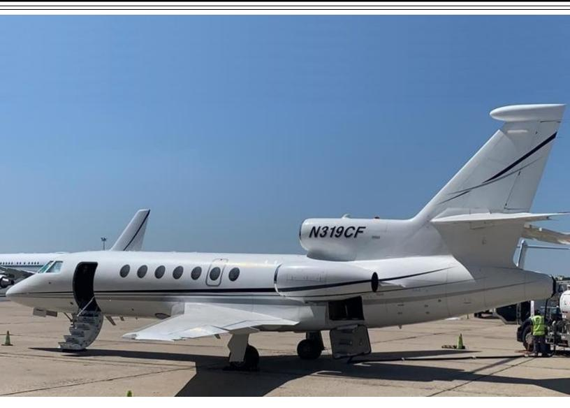
With three engines and leading edge slats, the Falcon 50EX offers superior range performance from fields as short as 4000 ft as well as comfortable direct transoceanic operations without ETOPS requirements. This SN 319 features upgraded FANS-1A and CPDLC avionics package. World class service and parts support is available through the manufacturer Dassault Aviation and many other independent facilities.
